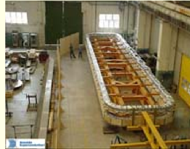
Central toroid under assembly
