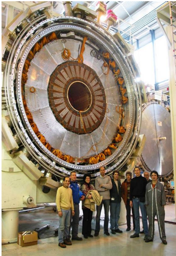
Endcap cryostat A before insertion of the FCAL
