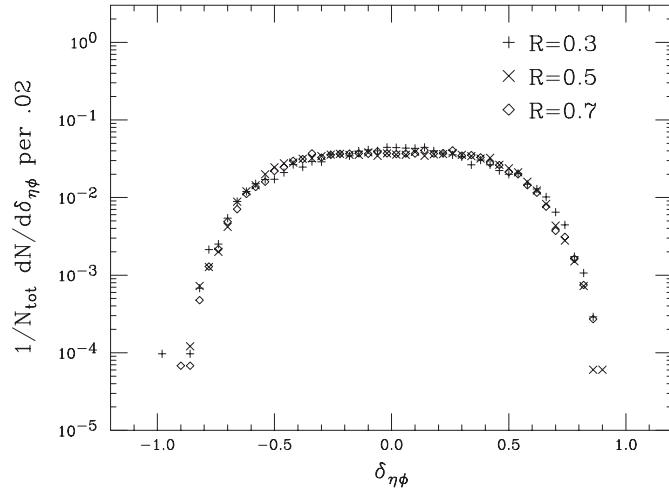
Fig. 17. The distribution in  $\delta_{\eta\phi} \equiv \frac{\sigma_{\eta\eta} - \sigma_{\phi\phi}}{\sigma_{\eta\eta} + \sigma_{\phi\phi}}$  using merged jets with cone cutoffs of 0.3, 0.5, and 0.7 from Sample 2.
