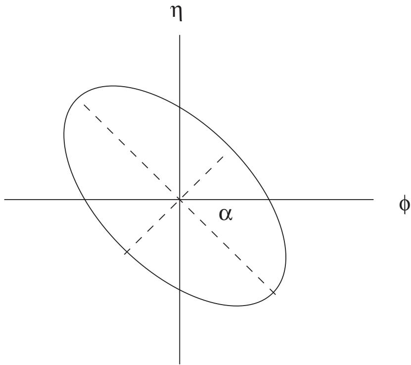
Fig. 7. Jet ellipse. Semi-major and -minor axes represent the square root of the second moment in  $\eta$  ( $\sigma_{\eta\eta}$ ) and  $\phi$  ( $\sigma_{\phi\phi}$ ).
