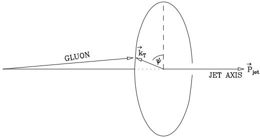
Fig. 4. Radiated gluons make an angle  $\psi$  with respect to an arbitrary direction in the plane perpendicular to the jet axis.
