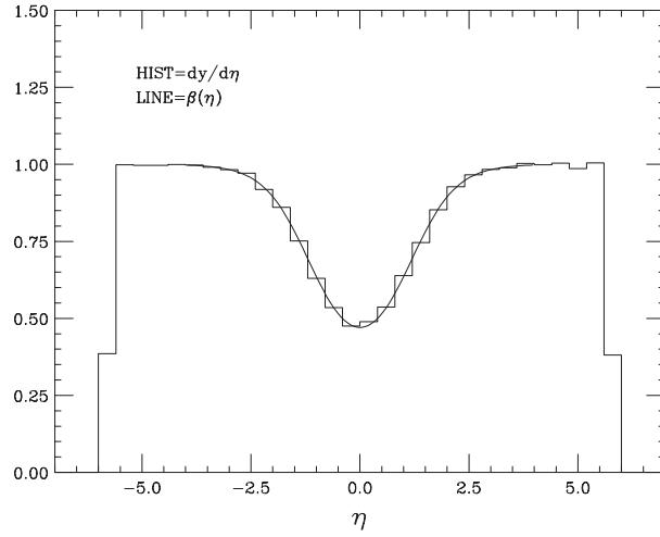
Fig. 3. The histogram shows  $dy/d\eta$  for pions generated uniformly in rapidity  $y$ , with fixed  $p_T = 0.5$  GeV/c. The smooth curve is the corresponding function  $\beta(\eta)$ .
