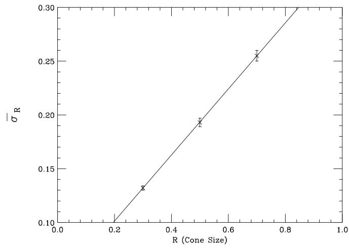
Fig. 6. Results of a Gaussian fit to distributions in  $\sigma_R$  as a function of the cone cutoff  $R$ . The straight line is from a linear fit to the points yielding  $\overline{\sigma_R} = (0.040 \pm 0.005) + (0.31 \pm 0.01) \cdot R$ .
